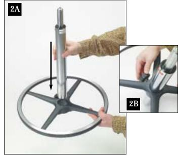
2. A. If your seat has a footrest, slide the footrest onto the bottom of center column and position it at the desired level. The footrest position can be adjusted later when the user is sitting on the seat. B. Tighten the footrest with the adjustable knob (turn clockwise) when in the desired position.
