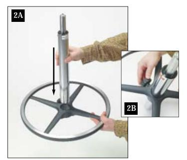
A. If your chair has a footrest, slide the footrest onto the bottom of center column and position it at the desired level. The footrest position can be adjusted later when the user is sitting on the chair. B. Tighten the footrest with the adjustable knob (turn clockwise) when in the desired position.
