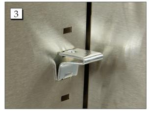
**Step 3.** When the top tab is snapped in, squeeze the bottom tab to the next lower hole, snapping it in place. Place shelf on clips.
