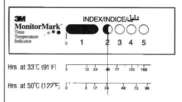
The above illustration shows how to use the runout indexes on the other side of this card to estimate the time a particular activated indicator has been exposed above its Response Temperature.
