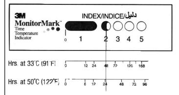
The above illustration shows how to use the runout indexes on the other side of this card to estimate the time a particular activated indicator has been exposed above its Response Temperature.
