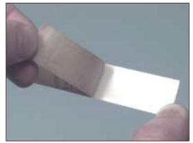
Attachment instructions: Peel the tan backing from the indicator until the white adhesive area is exposed. Press the white adhesive onto a clean, dry area by applying pressure to the indicator.
