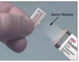
2. Pull the activation tab out and the attached barrier filmstrip will come with it. The indicator is now ready to monitor temperatures.
