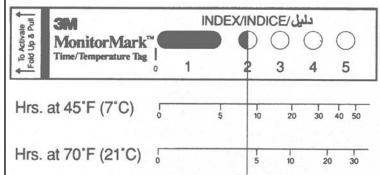
The above illustration shows how to use the runout indexes on the other side of this card to estimate the time a particular activated tag has been exposed above its Response Temperature.
