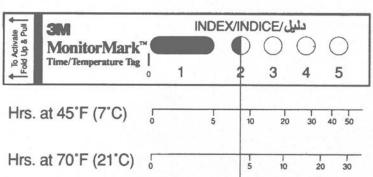
The above illustration shows how to use the runout indexes on the other side of this card to estimate the time a particular activated tag has been exposed above its Response Temperature.
