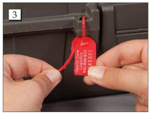
**Step 3.** To remove the seal, pull the tear-away rod away from the seal tab and away from the item being sealed.
