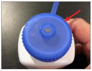
Bottle touching the Adapter Cap sealing surface as seen through the cap.
