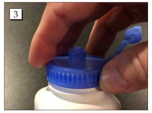
**Step 3.** Thread the cap onto the bottle. Be sure to screw the cap all the way down so that you can visually see the top sealing surface of the bottle contact the top of the Adapter Cap.
