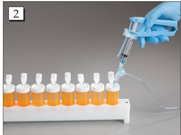
Step 2. Start at one end of the holder and fill the first vial. Continue moving from one vial to another until all of them are filled.
