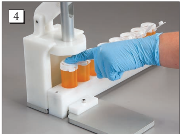
Step 4. Using your finger, push the tab down on the holder about to be sealed.
