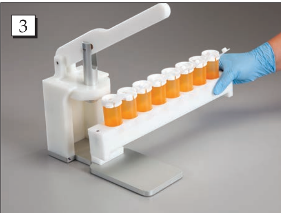
Step 3. Slide the holder into the channel base of the LUD Press. Make sure that the tabs are facing away from the press.
