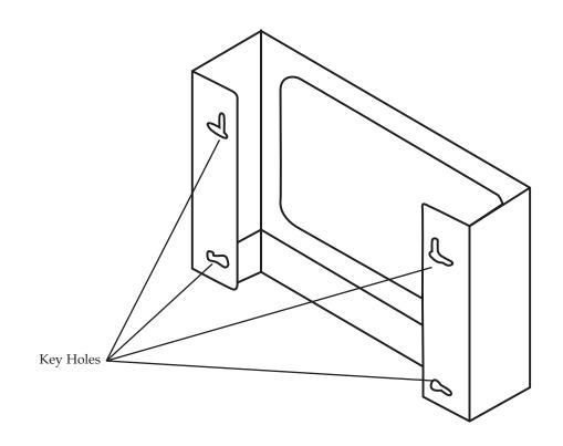
There are two way key holes for mounting purposes. This unit can be placed on the wall either horizontally or vertically.
