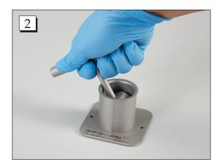
**Step 2.** Insert ball, press and move theT-handle side to side to pulverize.
