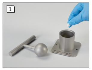
**Step 1.** Put the tablet in the removable stainless steel cup.
