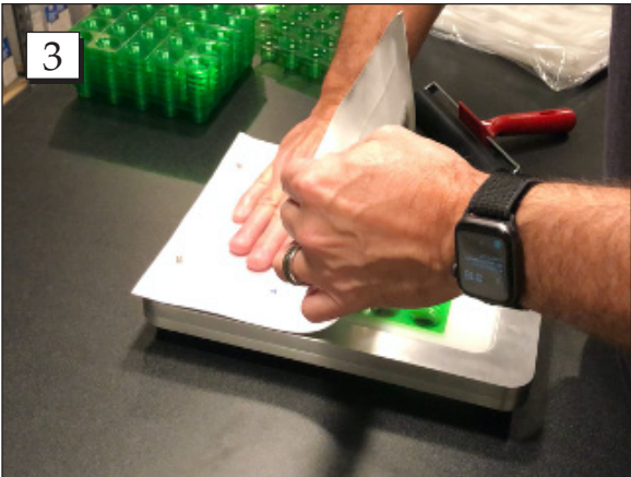
Step 3. Place the labels onto the locating pins and gently lay the labels onto the blisters.
