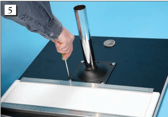
Step 5. Using a Phillips screwdriver, completely remove the four screws and washers from the center column plate on the underside of the workstation surface. Set the center column plate aside.
