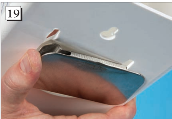
Step 19. With the flat side of the clip facing outward, feed one side of the clip back into the U-shaped groove on the back of the Glove Box Holder. Work the plastic on the holder onto the clip until both sides of the clip back are securely inside the U-shaped portion of the holder. This step may take several tries.
