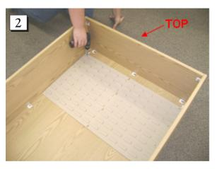
**Step 2.** Line the 1st panel up with the pre-drilled holes starting at the top, and use a screw and washer configuration to secure. (NOTE - make sure louvered panels are upright.)
