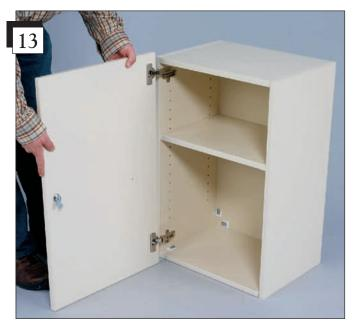
The door is ready to be attached. Position the door onto the side of the cabinet unit. The hinges should align with pre-installed hinge plates mounted inside of the unit.
