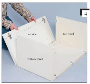
Attach the left side by aligning the pre-drilled holes with the connection fittings in the back, top and bottom panels.
