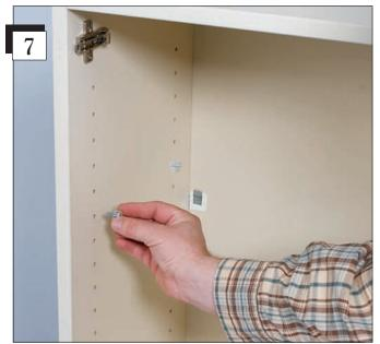
Stand your unit to the upright position. Decide the positioning of your shelves. Shelves are adjustable in 14" (32 mm) increments. Insert the clear plastic shelf pins in the back holes at your desired height. Once the back shelf pins are in place insert shelf pins into the front shelf holes at the same height as the back pins.
