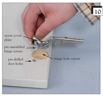
Begin by laying the door flat on the ground with the hinge hole cutouts (inside of door) facing up. With screw cover plate lifted, insert pre-assembled hinge screws into the pre-drilled door holes. There are two latches.
