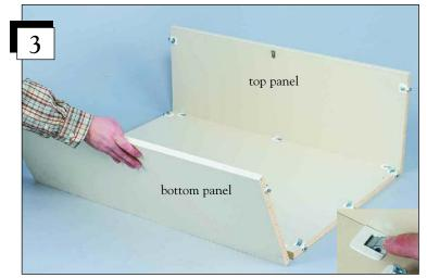
Attach the bottom panel by aligning the pre-drilled holes with the connection fittings in the back panel. Push the two panels together. Once together, press the fitting toggles down to secure.
