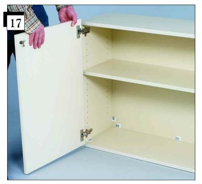
Doors are ready to be attached. Position the left door onto the side of the cabinet unit. The hinges should align with pre-installed hinge plates mounted inside of the unit.
