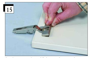
Once hinges are in place and flush against doors, press down on the screw cover plates to secure hinges to doors.
