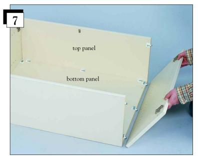
Attach the right side by aligning the pre-drilled holes with the connection fittings in the back, top and bottom panels. Push the panels together and press the fitting toggles down to secure.
