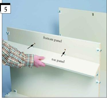
Locate the toe panel and attach to the bottom panel by inserting the connection fittings into the pre-drilled holes in the bottom panel.
