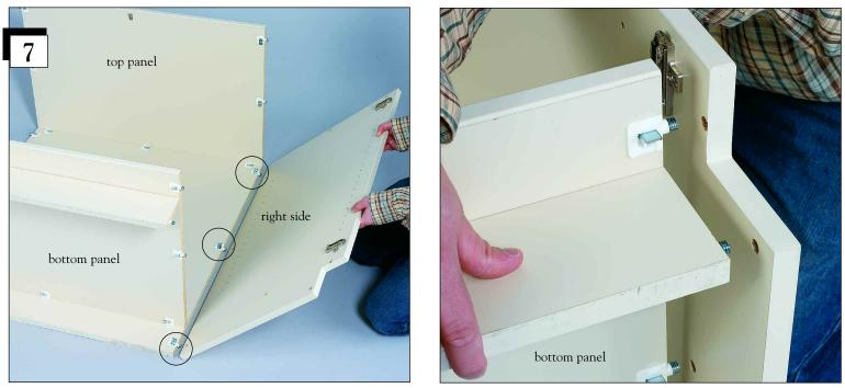
Attach the right side by aligning the pre-drilled holes with the connection fittings in the back, bottom and top panels.
