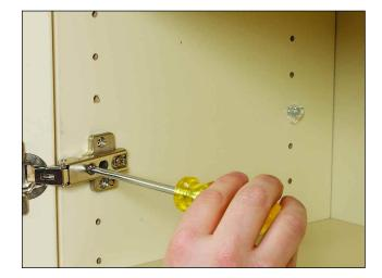
**The left adjustment screw provides depth adjustment:** Depth adjustment ... lets you bring any style of door into line with the vertical surface of the cabinet.
