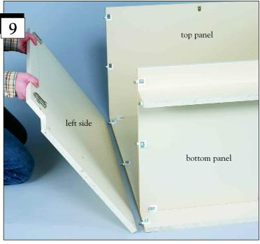
Attach the left side by aligning the pre-drilled holes with the connection fittings in the back, top and bottom panels. Push the panels together and press the fitting toggles down to secure. See step 8.
