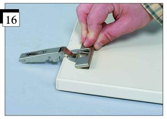
Once hinges are in place and flush against doors, press down on the screw cover plates to secure hinges to doors.
