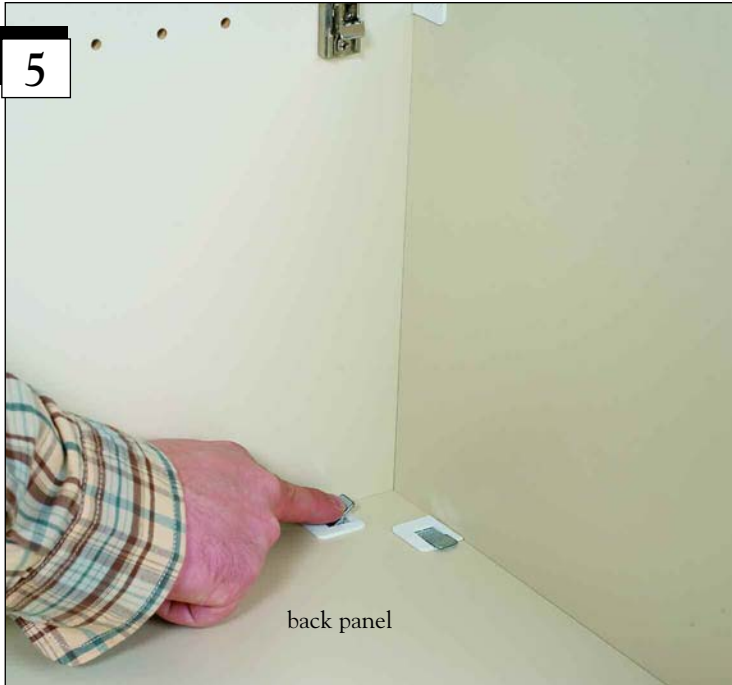
Push the panels together and press the fitting toggles down to secure.
