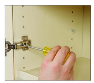
The left adjustment screw provides depth adjustment: Depth adjustment ... lets you bring any style of door into line with the vertical surface of the cabinet.
