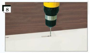
Using an 1/8" drill bit, drill the front hole in the template. You only need to drill a little bit into the shelf. CAUTION: Be careful not to drill all the way through the shelf. You may want to mark your drill bit with tape as a guide so you do not drill too far.
