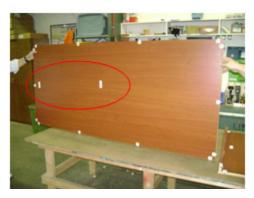
**Step 5.** With a helper, turn the center divider onto its side as shown - labels forward as shown.
