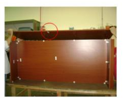
**Step 10.** Attach the Right Side Panel to the Center Divider as shown - NOTE: make sure the label is on the same side as pictured.
