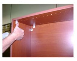
**Step 14.** Press the four fitting toggles down as shown - the other is on the other side of the Center Divider. The other two are on the opposite end.
