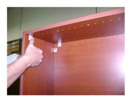
**Step 11.** Press the four fitting toggles down - the other is on the side of the Center Divider. The other two are on the opposite end.
