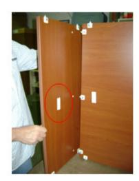
**Step 8.** Attach the Top Panel to the Center Divider opposite the Toe Panel Bottom as shown - label on the same side as shown.
