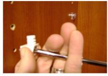
**Step 18.** Once the clear back shelf pins are in place, insert the front white shelf blocks into the front shelf holes and tighten with a Phillips screwdriver. Repeat steps 17 and 18 on the opposite side.
