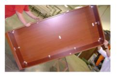
**Step 16.** With a helper, move the unit upright with the Toe Panels on the floor.
