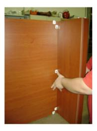
**Step 7.** Press the three fitting toggles down to secure.
