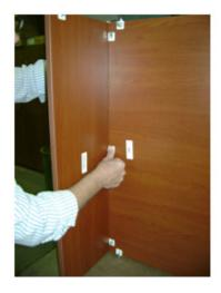
**Step 9.** Press the three toggle fittings down to secure.
