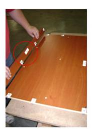
**Step 3.** Repeat steps I and 2 to attach the second Toe Panel on the opposite side of the Bottom Panel.
