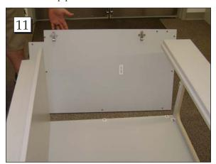
Step 11. Attach the left side by aligning the predrilled holes with the connection fittings in the back, top and bottom panels.
