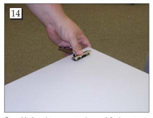
**Step 14.** Once hinges are in place and flush against doors, press down on the screw cover plates to secure hinges to doors.
