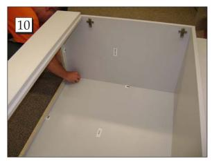
Step 10. Push the panels together and press the fitting toggles down to secure.
