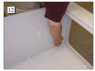
Step 12. Push the panels together and press the fitting toggles down to secure.
