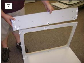
**Step 7.** Attach the front panel to the inside of the
