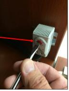
**Step 1.** Use a straight head screwdriver to preset cabinet to the desired temperature. Close the door and allow the unit to warm for 24 hours.
