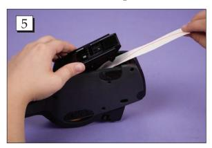
**Step 5.** Pull the tail out and close the bottom assembly.
