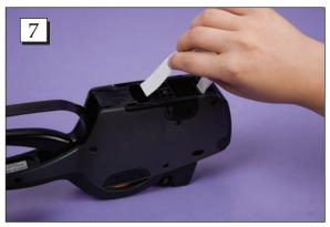
**Step 7.** Feed the tape through the feed drive wheel on the side closest to the handle.
