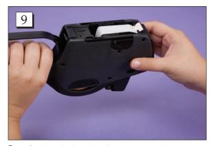
**Step 9.** Click the handle of the gun several times to progress the tape through the gun.
