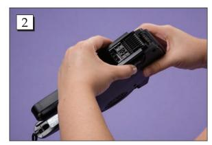
**Step 2.** Press both side cap locks to release the bottom assembly.
