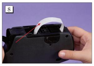
**Step 8.** Be sure to remove the labels on the outside of the gun. Otherwise they will get clogged up when the tape advances through the gun.
