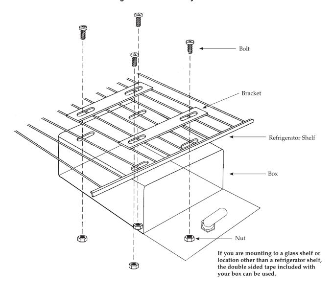
This box was designed to be attached to wire grid type refrigerator shelves. If possible remove the refrigerator shelf unit on which the box is to be installed. Tools required: a 7/16" wrench or a socket and a Phillips screwdriver.
