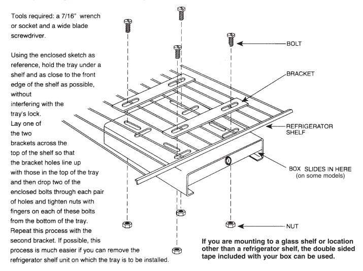
Put the wrench or socket on each nut from the bottom of the tray and tighten with the screwdriver from the top. Do not completely tighten all the bolts/nuts until you have determined the final position. Note: these are special nuts that require a fair amount of effort to install...however, once installed they can not be loosened without access to the bottom of the tray.
