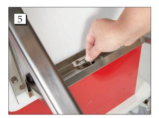
**Step 5.** Latch bottom retention clasp to lock the legs in place.
