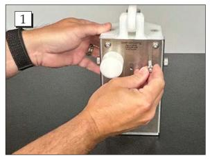
**Step 1.** Remove the <sup>1</sup>/<sub>4</sub>" Socket Head Cap Screw from the back of the unit.
