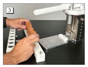
**Step 3.** With the top of the carrier removed, place the Easy Fill Vials onto the base.
