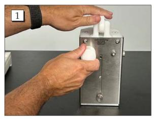
**Step 1.** Remove white the Anvil Insert from the back of the unit.
