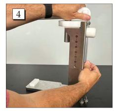
**Step 4.** Adjust the height of the top until the proper position number lines up with the threaded hole. Tighten the thumb screw once at the desired height.
