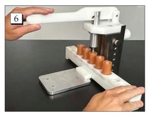
**Step 6.** Place the Easy Fill ball over the sealing hole in the vial, and gently press the ball into place.
