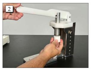
**Step 2.** Thread the white Anvil Insert into the bottom of the Anvil.
