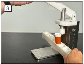
**Step 3.** For Tamper Tuf Vial "Unassembled", place the Vial with Cap on top into the carrier and under the press. The carrier should slide smoothly from left to right. For Tamper Tuf Assembled skip to step 5.
