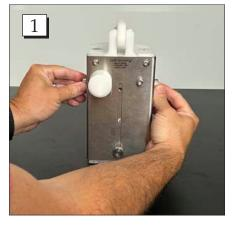
**Step 1.** Remove the thumb screws from the right and left side of the unit.
