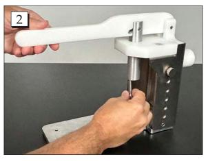
**Step 2.** Thread the ¼" Socket Head Cap Screw into the bottom of the anvil as far as it will go.
