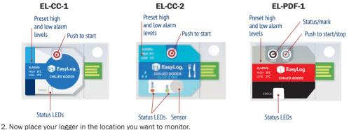
Once logging, pressing the  $\odot$  button will light up an LED only on PDF, CC flashes, to give a quick indication of the status. It will also add a marker to the data to show that you have checked it. No alarms will be triggered in the first 30 minutes to allow the logger to settle at the monitored conditions periodically.
