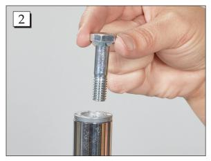
**Step 2.** Manually screw the desired foot (Standard or Plate Foot) into each nut.
