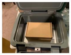
**Step 3.** Place one USB Probe Data Logger that has been chilled to approximately 40°F inside of a cardboard box.
