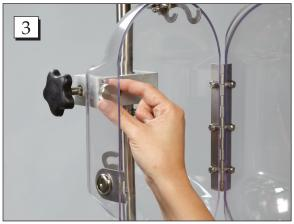
**Step 3.** Tighten the locking wheel on the inside of the pod.
