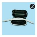
Loop the right end of the cable under the suppressor and back up again laying the cable along the center of the suppressor.
