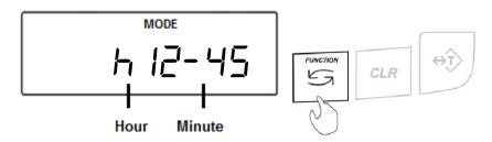
4. Once the minutes and hours are confirmed the screen will switch automatically to the time of day selection. Select "###" or "###" by pressing the T key.
