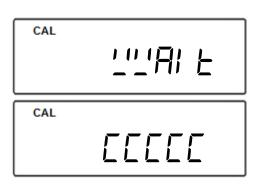
10. When calibration has ended the scale will display Pr\_On. Toggle the calibration switch in the rear of the scale back to its original position.
