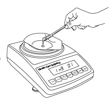
7. Once a desired weight is displayed press the T key to store the ingredient in the scale's memory.
