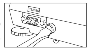
Warning: Do not attempt to screw the flush sealing screw all the way in. Stop when the screw is flush with the casing of the scale.
