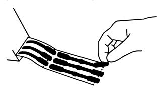
**Step 3**: Press ends firmly to affix the seal to the device.
