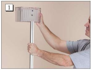
**Step 1.** Slide the T-Nuts on the label dispenser onto the pole.
