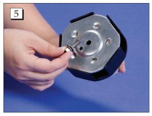
**Step 5.** Insert the screw through the hole on the cover plate into the pole adapter and thread the screw in three turns.
