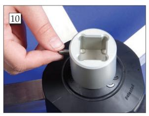
**Step 10.** Back the set screw out of the pole adapter.
