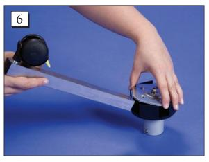
**Step 6.** Tilt the cover plate up and insert a leg section with the open hole in the leg facing upward toward the cover plate.
