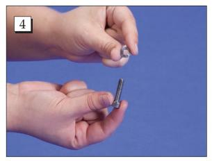
**Step 4.** Place a lock washer first followed by a flat washer over the screw.
