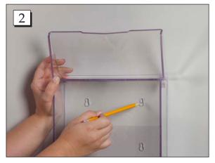
**Step 2.** Lift the lid and use a pencil to mark the drill holes.
