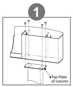
Attach selected accessory to the column using (4x) screws included with stand. Tighten.
