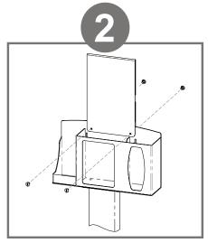
To mount a sign holder on an accessory without a lid, sandwich the accessory top between the holder, lining up holes. Attach using (2x) barrel screws included with sign holder.
