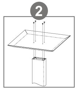
Use Phillips screwdriver to secure base to column with (4x) screws (10-32 x 5/16").
