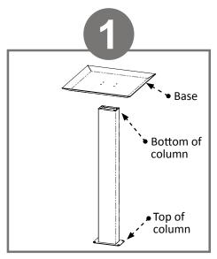
To secure base to column, turn column upside down (with top plate down) and place base inverted, as shown, on column.
