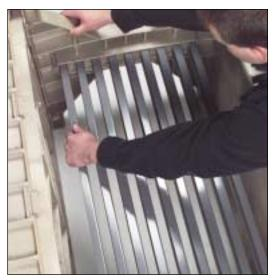
19. Place the remaining rails into the molded openings. It is easiest to put one side of a rail in one end of the cart and then angle the rail until it will fit into the other end. When all rails are in place, connect the end tightly to the shelves. You may need to tap the cart end with your rubber mallet to get a tight fit.
