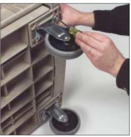
**16.** Move to the bottom shelf. Align the shelf and end holes and attach the remaining 2 casters using short screws and your screwdriver.
