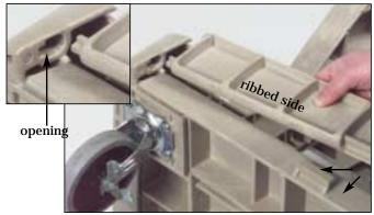
12. Connect the bottom panels to the bottom shelf (ribbed side facing out and notches at the bottom) by inserting the small notches into the openings in the cart. Slide the flat notched sections into the clips on the side of the shelf. To put panels on both sides of the shelf, the cart may need moved to the upright position.
