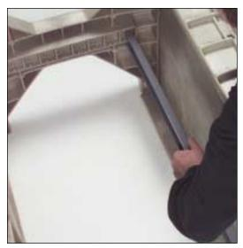
**18.** Place the hanging rails flat side down into the molded holes in the ends of the cart . Keep pressure on the end that is slightly attached so the rails do not fall out of the molded holes.
