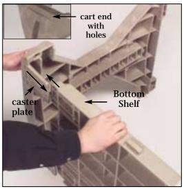
1. Insert the notches on the bottom shelf into the large grooves at the bottom of the cart end that has holes for the handle. The bottom shelf is the shelf with the smaller notches. The caster plates on the cart end should be under the shelf.
