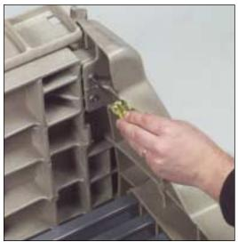
**20.** Align the holes from the cart end with the holes in the top shelf. Insert the short screws and tighten them.
