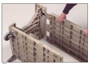
**7.** Lay the cart on its side. Insert the notches on the top shelf into the large grooves at the top of the cart end. The top shelf is the shelf with the longer notches.
