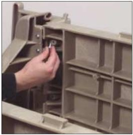
**9.** Insert a long screw into the hole next to the screws you just inserted and tighten it.
