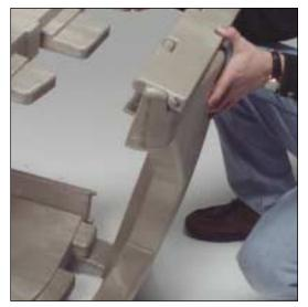
17. Turn the cart to the upright position. Slightly attach the second cart end (with clips on top) to the top and bottom shelves by inserting the notches on the shelves into the cart end grooves. Make sure that the cart end caster plates are under the bottom shelf. Do not connect them tightly. Turn the cart on its side.
