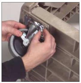
**3.** Using the shorter screws, place them into the aligned holes.
