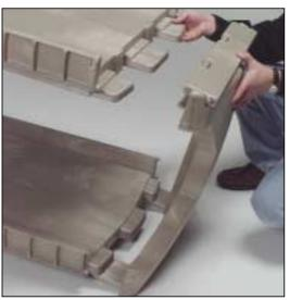
**14.** Turn the cart to the upright position. Attach the second cart end to the top and bottom shelves by inserting the notches on the shelves into the cart end grooves. Make sure that the cart end caster plates are under the bottom shelf.
