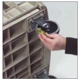
**21.** Move to the bottom shelf. Align the shelf holes and the caster plate holes in the cart end and attach the remaining 2 casters using short screws and your screwdriver. Your finished.
