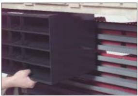
Cassettes hang from the rails using suspension straps.
