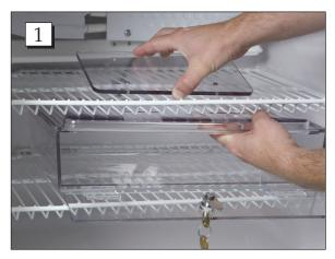
**Step 1.** Place hand inside box and hold into place while placing retention plate on top of refrigerator rack.
