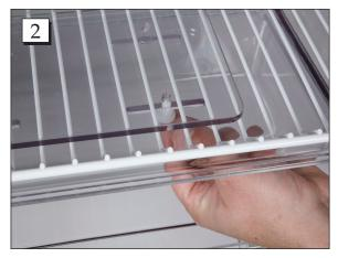
**Step 2.** Thread screw from the inside of the box through the rack into the retention plate - (trap refrigerator rack between box and retention plate).
