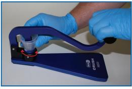
4. Between each crush, release the handle to the start position (you do not need to lift the handle up) and gently turn the cups. The pills will crush with the spring/twisting motion of the anvils.
