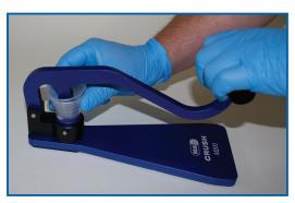
**3.** Apply gentle pressure to the handle. This alone will crush the pills. You do not need to pound or hammer!
