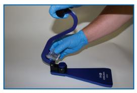
Place pill(s) into a crusher cup and then cover with a second crusher cup. Slide the cups on the handle anvil. We recommend 1 oz. (30 mL) plastic cups.
