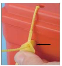
Pull the seal as tight as possible while guiding the dome of the seal into the bottom hole on the box.
