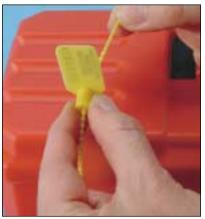
Pull the tail of the seal through the locking dome.
