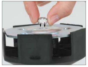
4. Place the locking spacer into the center opening of the clamp disk. The teeth should fit against the disk.
