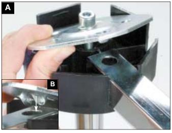
(A) Lift the clamp disk up and slide one of the feet with electrically conductive casters into the 5-footed plastic midsection. (B) Align the groove on the clamp disk with the hole in the foot and push the clamp disk down until they snap together.
