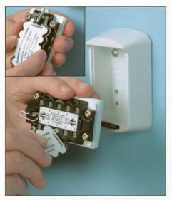
4. Remove the white card from the back of the front door and use the pointed edge to set your combination. *Holding the combination pad in the horizontal position*, set the combination by turning the desired numbered push buttons clockwise to the on position.
