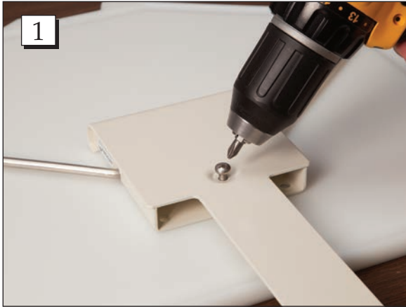
Step 1. Rotate Wall Bracket assembly to remove the cover screw and cover.
