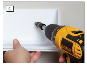
**Step 4.** Loosely drive the screw into the desired location on the wall or cabinet. (Screws are not provided.)
