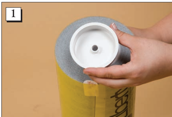
Step 1. Gather one end cap and the tacky roll. Place the end cap in the open end of the tacky roll.
