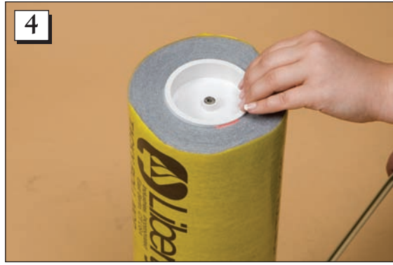
Step 4. Place the remaining end cap in the open end of the tacky roll. Be sure to line up the axle with the hole in the bottom of the end cap.
