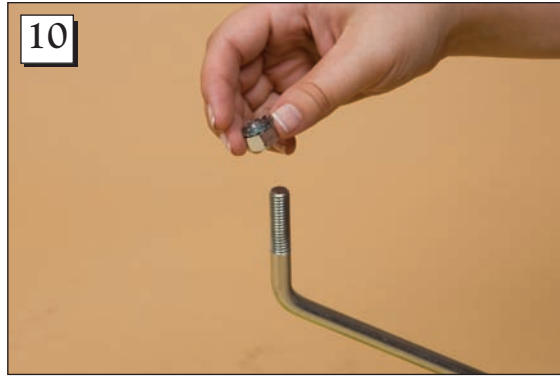
Step 10. Place the lock nut on the end of the axle with the prongs facing up.
