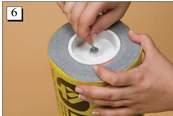
Step 6. Place both the screw and washer into the end of the axle.
